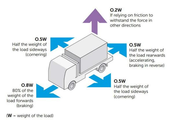
If a load is restrained to meet these Performance Standards it will not fall off or affect the stability of the vehicle under expected driving conditions. This includes emergency braking and minor collisions.
